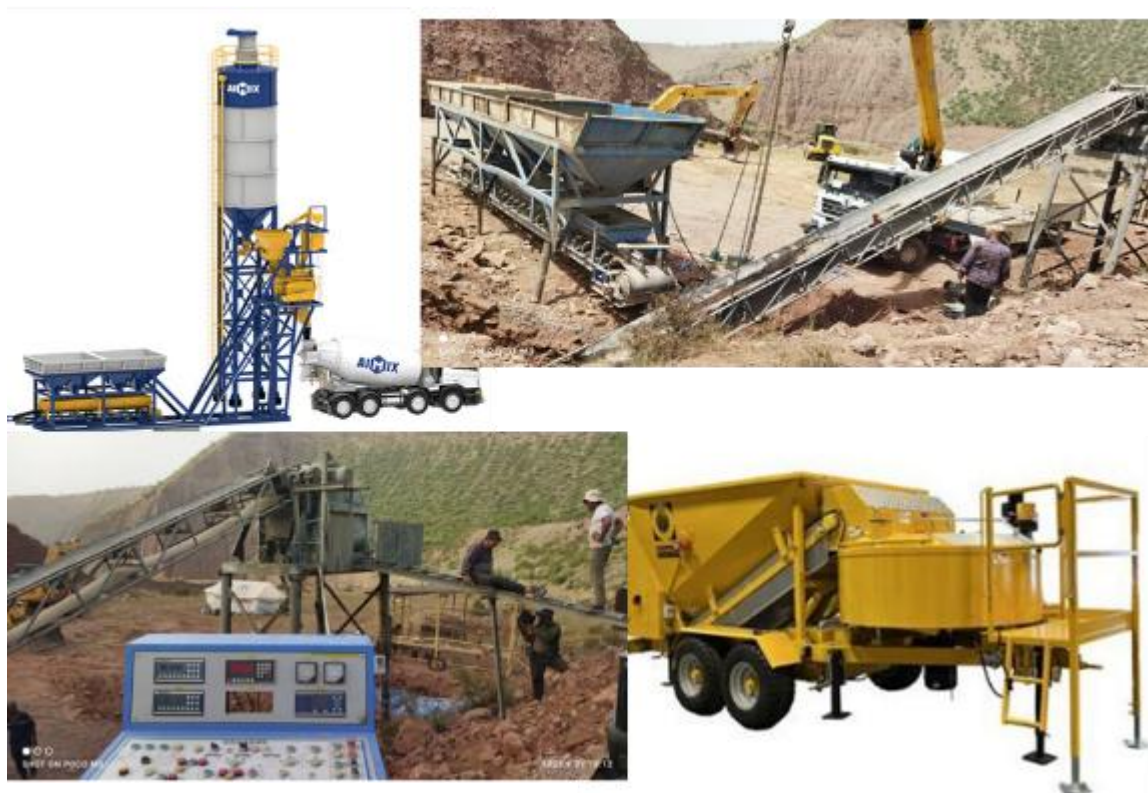
Figure 12. Typical Small Batching Plants
